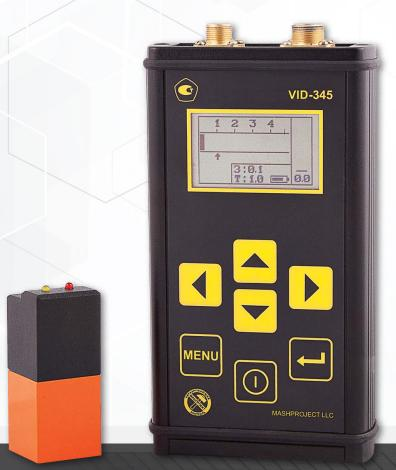
The magnetic-eddy-current flaw detector VID-345 is intended for detecting and measuring of depths of stress-corrosion fractures in ferromagnetic structures as well as fractures under the insulating coating and/or corrosion layer.
