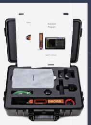
The EM4000 electromagnetic acoustic thickness gauge is capable of connecting to a tablet, smartphone or another device based on the Android OS. This allows expanding the thickness gauge features, analyzing A-scans, B-scans, working with strobes, selecting a thickness measurement mode, signal processing parameters, etc. The EMA thickness gauge can be connected to a tablet either wirelessly via Bluetooth or using a USB cable.
